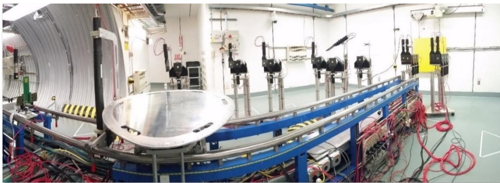
Fig.3. Galactic Cosmic Ray Simulator at Brookhaven National Lab (US). A GCR simulator uses new technology that allows to test multiple ion beams at one time to accurately represent the radiation conditions that an astronaut is exposed to in a spacecraft. Studies on the effects of radiation on CNS and other endpoints has been done only on ground at the accelerator facilities or through simulations. (Photo Courtesy of NASA).
