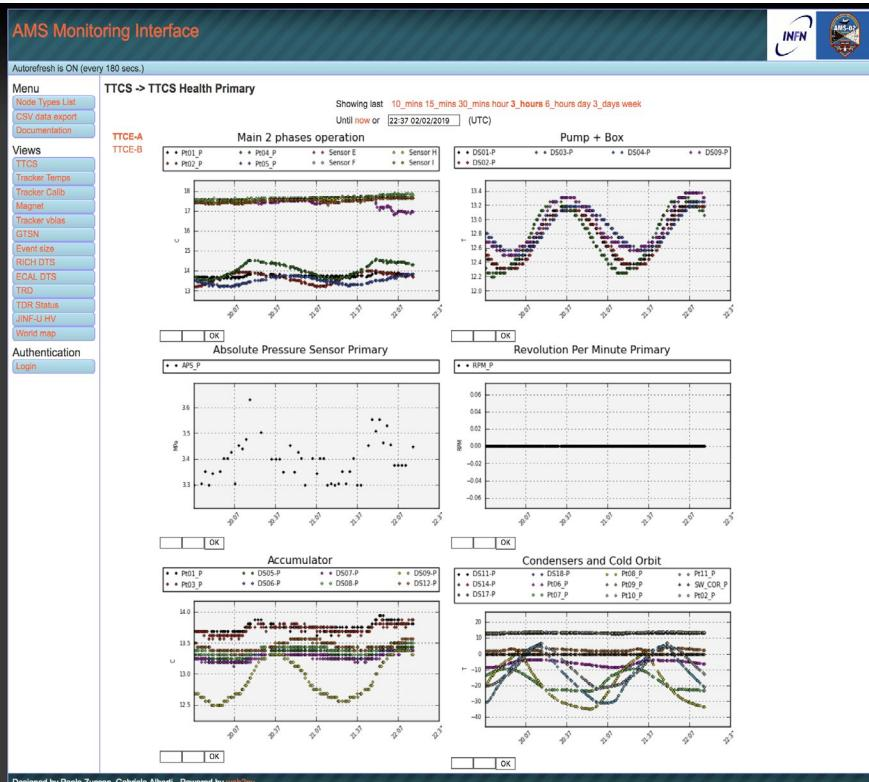
TTCS spike alert : for prompt alert on anomalous pump RPM
