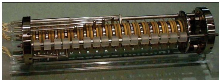
Figure 1. Electrostatic forces generated by this apparatus work in concert with a magnetic field to create a Penning trap. Researchers at NIST will use the device to trap and count the protons emitted from a collimated beam of decaying neutrons. By simultaneously monitoring the flux of neutrons through the trap, the researchers should be able to measure the neutron lifetime to within 0.1% accuracy. (Photo courtesy of Geoffrey Greene.)
