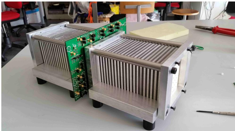
FIG. 2: Test prototype for the light readout system of the calorimeter based on SiPM embedded in the shashlik module.
