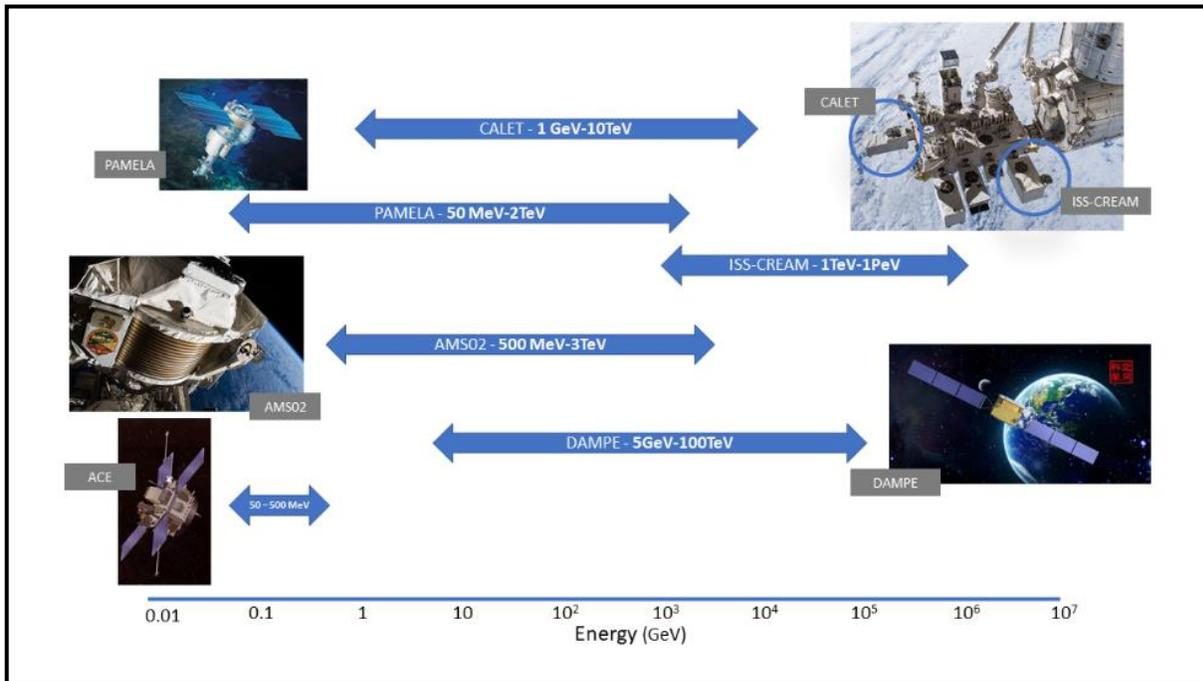
Fig. 3. Measurement's energy range of some Cosmic Ray Detectors operating in space
