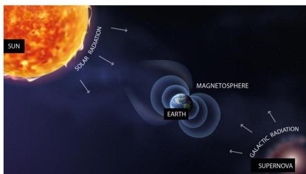
Fig. 1. The Space Radiation Environment is a complex mixture of radiation species coming from outside the solar system, generated by the sun and trapped in the Magnetosphere (credit IAEA)
