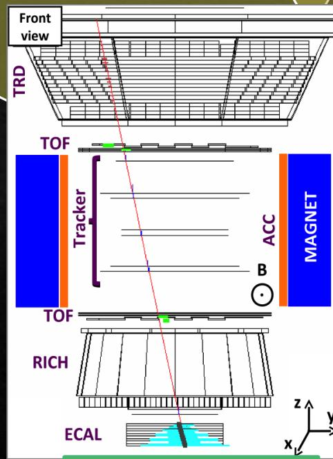
Signature of a 4GeV electron in AMS detector
