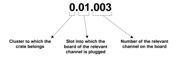
Fig. 4.2 - Complete Channel address
