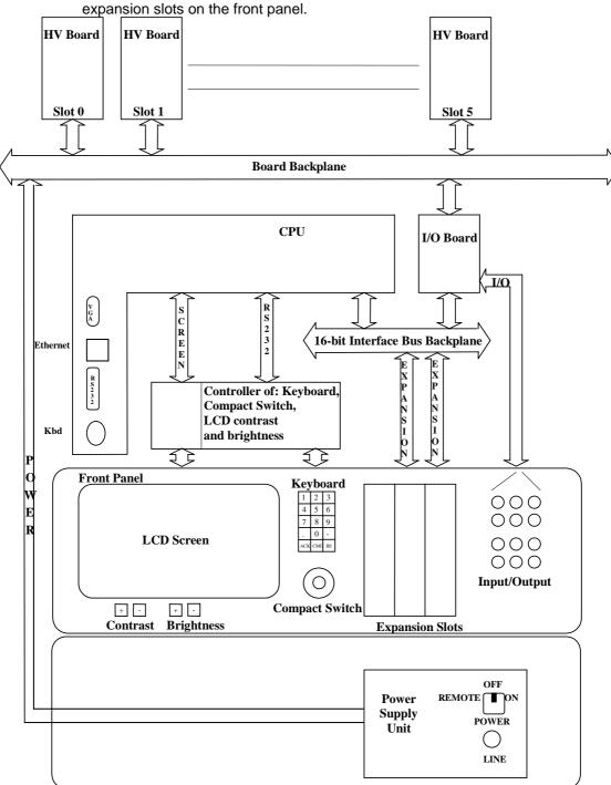
Fig. 2.2 – Block diagram of the functional parts of the SY2527 system
