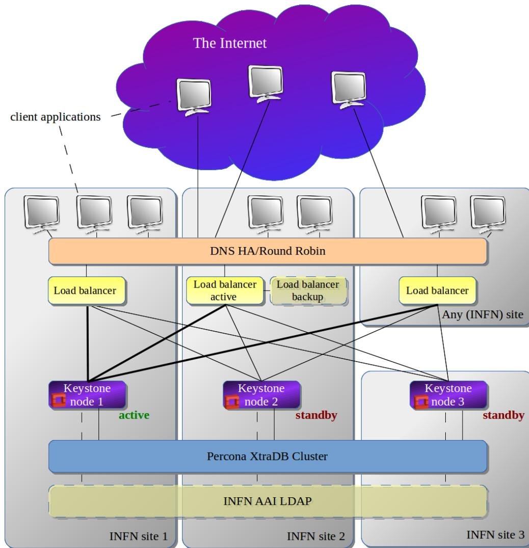
HAProxy is used as a load balancer and HA provider. One or more HAProxy nodes contact the active Keystone server, falling back to the second and to the third should the checks they periodically perform on the active authentication server fail.
