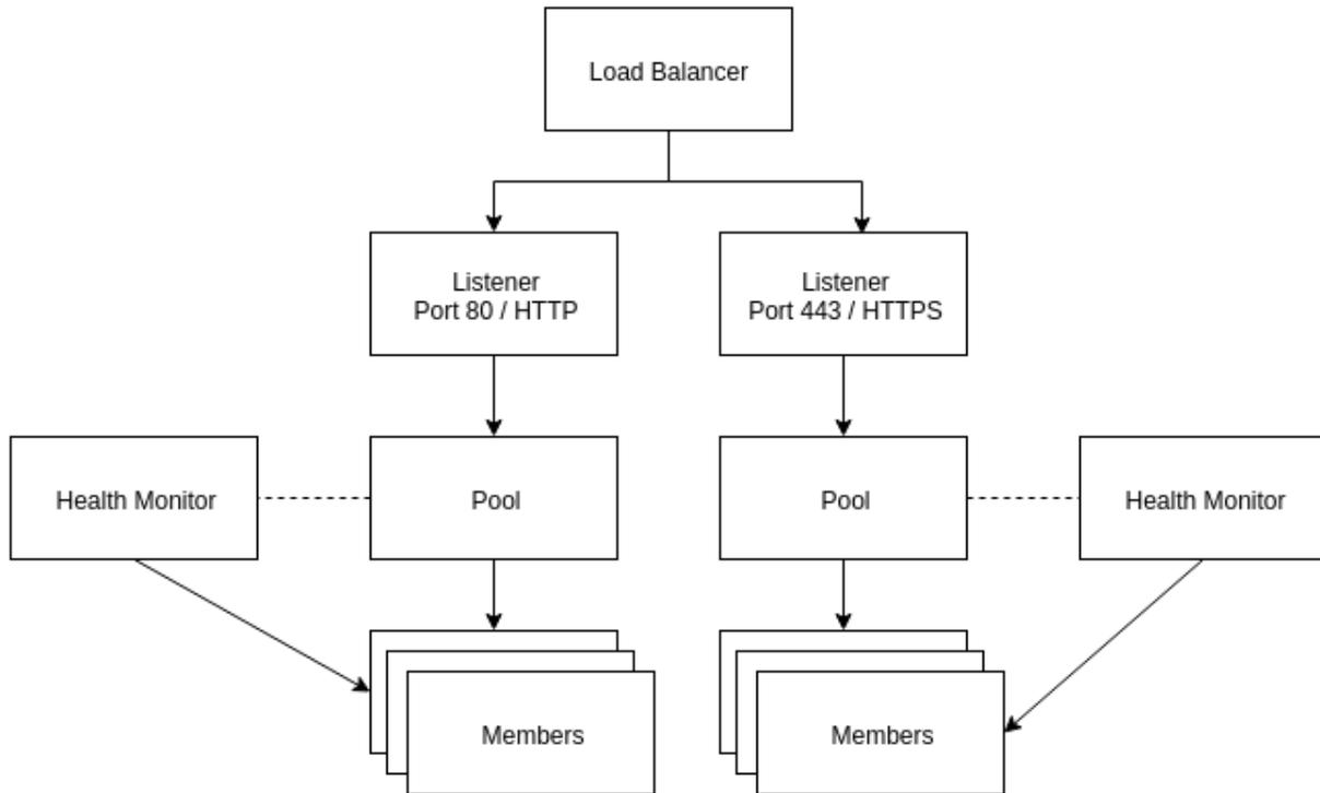
**Load balancer** The load balancer occupies a neutron network port and has an IP address assigned from a subnet.
